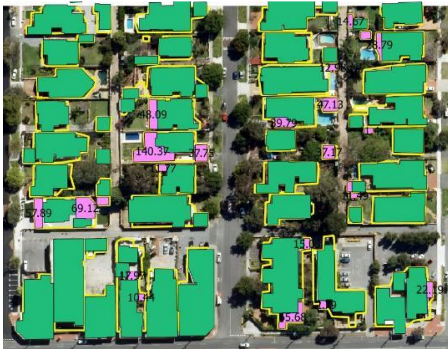
Figure 2. Green: Old data; Yellow: Automated result; Pink: Change detection with change figures in sq meter
