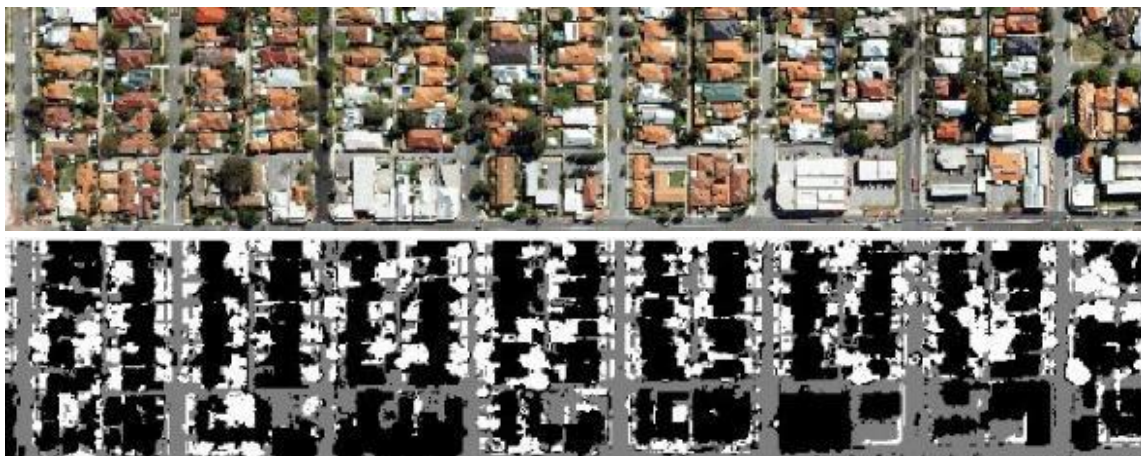
Figure 1. Building footprint detection through deep learning. Top: Original image. Bottom: Image classification result where black colour represents the buildings.
